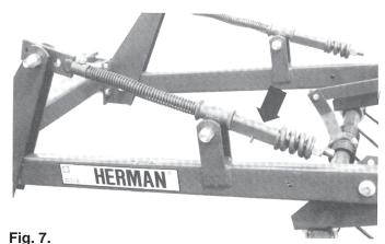
7a. Lock-up clip shown installed (see arrow) to hold harrow up in a raised position.
